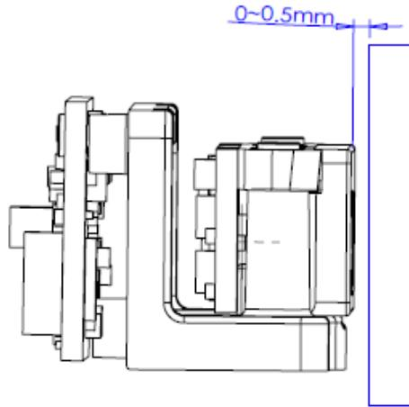
If the window is required to be in a tilted position, the above distance requirements should be met and tilt angle should ensure no reflections back into the lens.
