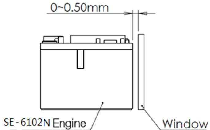
If the window is required to be in a tilted position, the above distance requirements should be met and tilt angle should ensure no reflections back into the lens.
